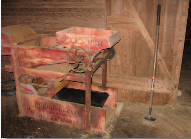
Russ Miller's restored Clipper seed cleaner which he uses to clean his hull-less oats.
